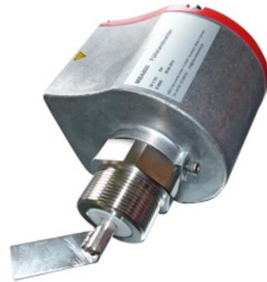
Direct drive without gearbox, powerful motor with miniature paddle, selectable pre-set parameter combinations for universal use – those are the main features of the new MBA800 rotating paddle series for level measurement. The adjustment of the different motor control parameters can be adapted for different types of bulk goods and their behaviour in the respective application.
